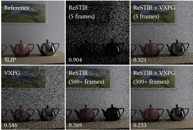
Fig. 10. Image quality comparisons for our approach (VXPG), ReSTIR GI [Ouyang et al. 2021] (ReSTIR), and their combination (ReSTIR + VXPG). We also show the effect of the ReSTIR variants after both small and large amounts of temporal reuse. The top row represents images captured after 5 frames of temporal reuse, while the bottom row corresponds to images captured after more than 500 frames with M\text{-cap} = 20 .
